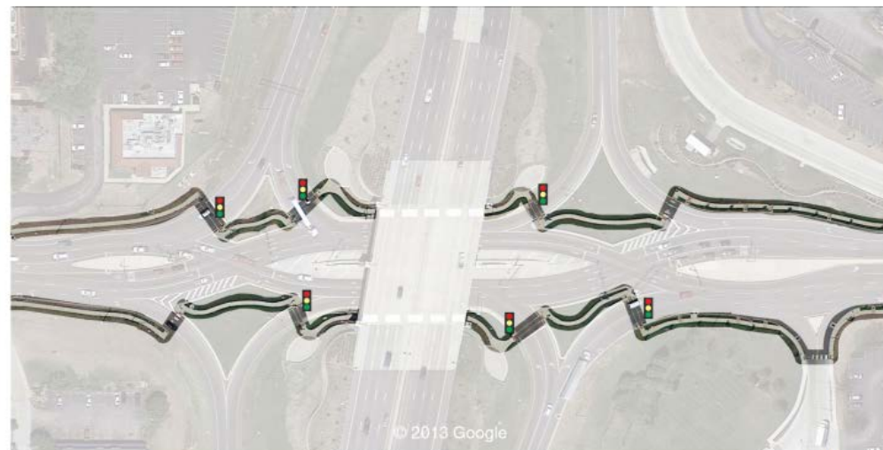
Exhibit 3-6. Pedestrian facilities on outside of DDI (Maryland Heights, MO). (26)
