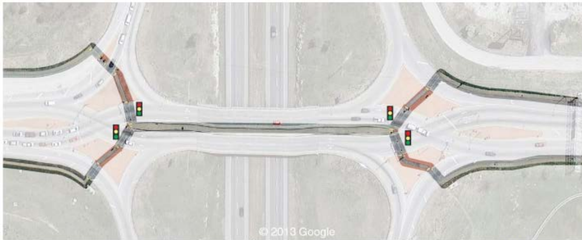
Exhibit 3-5. Pedestrian facilities in center of DDI (Springfield, MO). (26)
