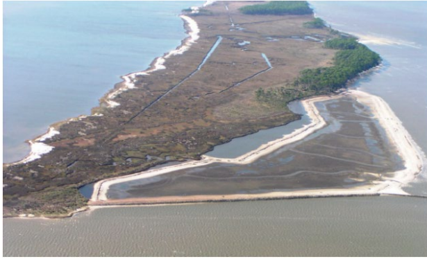
Figure 3. Deer Island with channels and marsh grasses planted (pre-Hurricane Katrina, spring 2004) (Roth et al., 2012).
