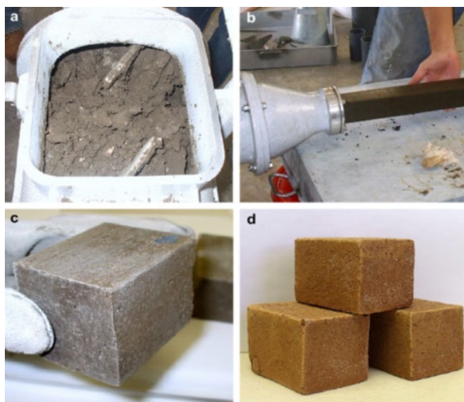
Figure 17. Photos. Laboratory-scale brick production: (a) raw material mixing, (b) extrusion of a brick column, (c) dried brick, (d) fired bricks (Mezencevova et al., 2012).
