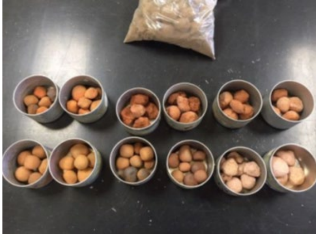
Figure 14. Photo. Lightweight aggregate made from dredged material in Ohio (Liu et al., 2018)
